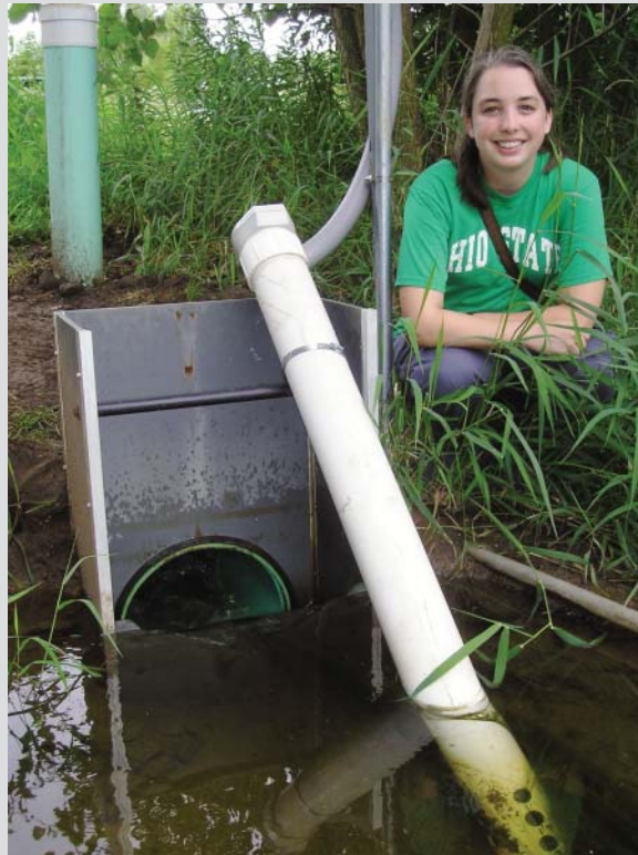
Figure 4.9 Control structures such as the V-notched weir shown here can be used for measuring surface water flow in small streams into or out of wetlands. (Photo by W. J. Mitsch)
